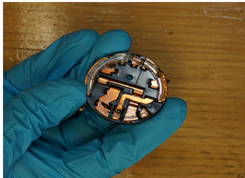
The corroded switch
